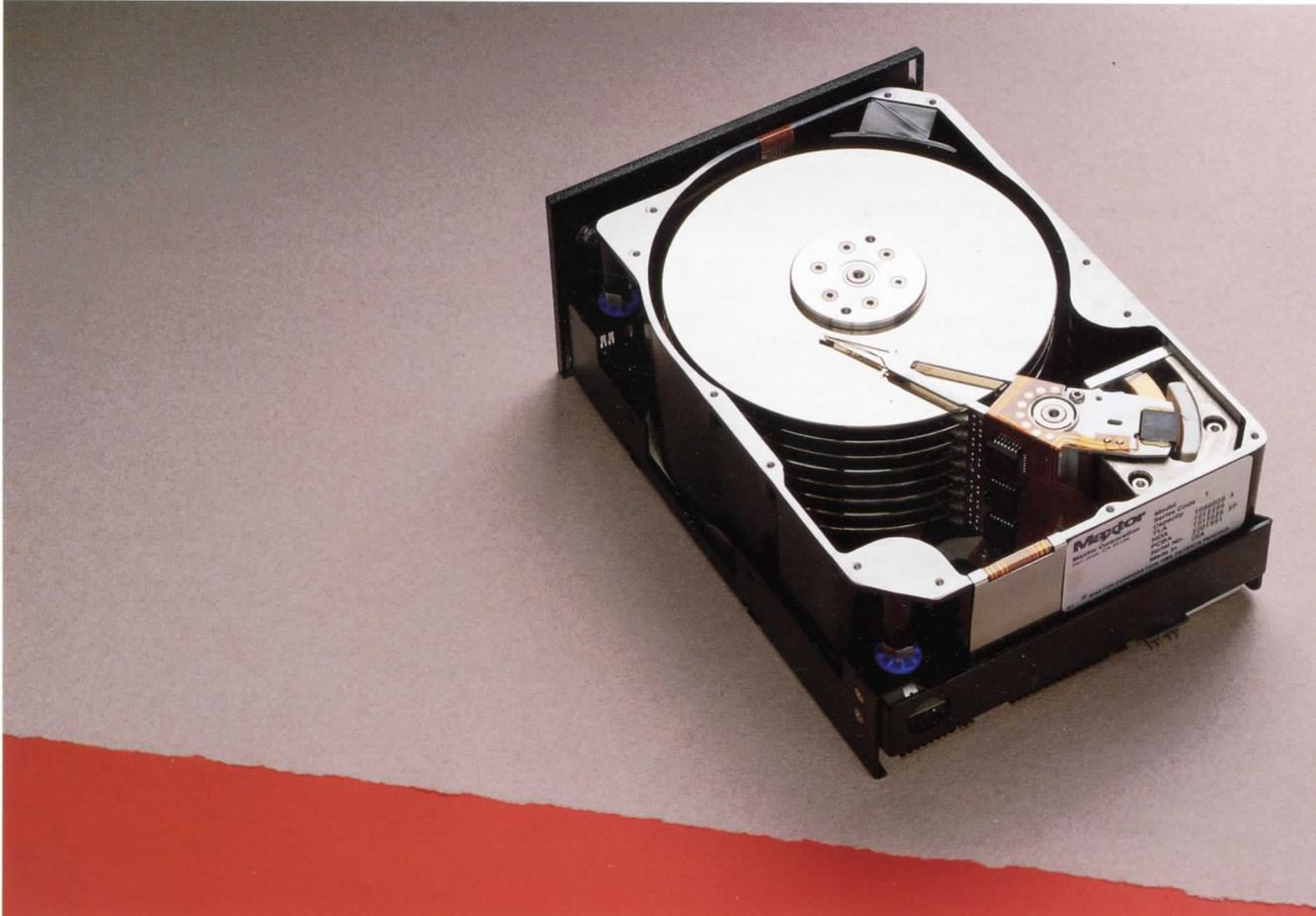
This high-capacity 5 1/4-inch disk drive incorporates the ESDI high-performance standard interface. Fast seek times of 16.5 and 14.5 msec provide the performance necessary for today's system applications. A 15 Mbit/sec transfer rate, and status and configuration reporting across the interface are included in the benefits of this high-capacity, high-performance disk drive family. The XT-8000E family offers size and cost reduction opportunities relative to larger-sized, high-capacity disk drives.
