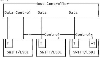
Total control cable length must not exceed 10 feet (3.00m). Each data cable length must not exceed 10 feet (3.00m).
