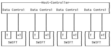
Each control cable length must not exceed 10 feet (3.00m). Each data cable length must not exceed 10 feet (3.00m).
