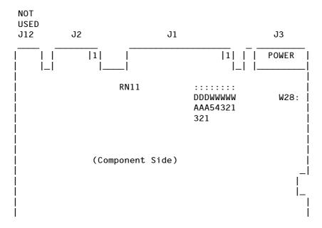
The Interface Terminator factory installed at RN11 will provide proper termination for the interface lines. When daisy-chaining multiple drives, leave the terminator installed only in the last physical drive on the daisy chain cable; remove the terminator from each of the other drives. In most PC/AT installations, the C: drive is actually at the end of the cable and should retain the terminator.
