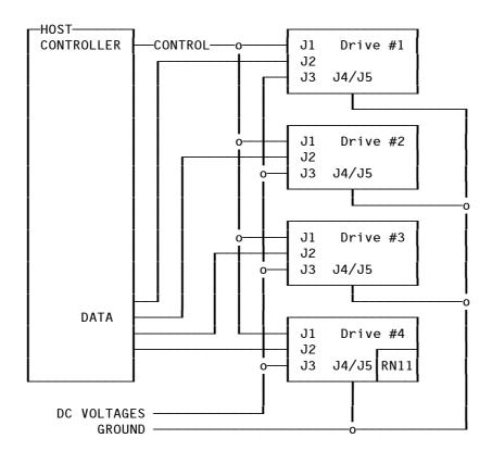
Interface Terminator RN11 is installed ONLY in the last physical drive in the control chain.
