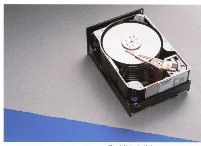
This reliable family of high-performance 5.25-inch disk drives incorporates the ESDI high-performance standard interface. Fast seek times of 16 through 14 msec provide the performance necessary for today's system applications. A 10 Mbit/sec transfer rate, status and configuration reporting across the interface and NRZ data transfer are among its many benefits. The XT-4000E family offers size and cost reduction opportunities for existing systems using larger-sized, high capacity drives.
