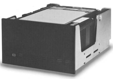
The Micropolis 1518 high performance 5 1/4-inch Winchester disk drive offers 1.53 gigabyte capacity and an ESDI interface in a full-height form factor.
